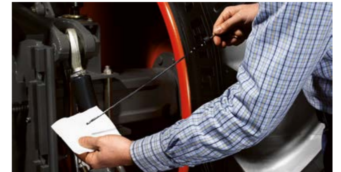
It's easy to check the transmission oil level at the rear.
